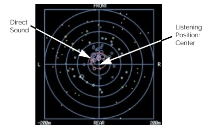
Virtual sound sources are blue or white Distribution of Sound Field Data Round scale is a reflection strength.
