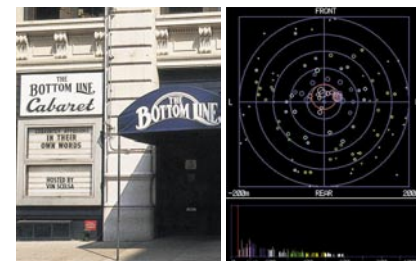
Imaginary Sound Source Distribution of Sound Field Data EFCT TRIM 0 dB INIT.DELAY 30 ms ROOMSIZE 1.0 LIVENESS 5 S. DELAY 5 ms* * Dolby Digital/DTS Input
