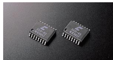
High-Quality Digital Volume Devices (Crystal Semiconductors' CS3310 LSIs)
