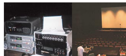
DSP Uses Actual Sound Field Data Single Point Quad Miking array precisely measures the acoustic patterns of a sound space and are placed on the same plane or in proximity to each other to capture pulsive sounds, and their impulse responses are recorded.
